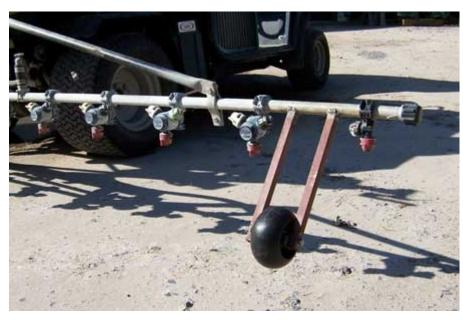
Our sprayer is very low to the ground and after breaking off so many nozzle holders after they make the turn into the rough, I made wheels on the booms. It only cost about thirty dollars to make. Wheels ordered through Napa, half inch round steel for the shaft for the wheel. 3/4 inch square tubing attached to the boom.
